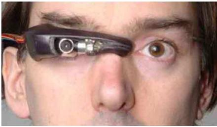
**Figure 9: New injection moulded design.** From this figure we see how the camera has been effectively mapped to the position of the human eye by the EyeTap configuration as outlined in Figure 1.
