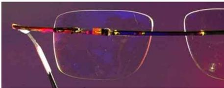
**Figure 10: In one design prototype, the computational element of the eyeglasses is incorporated into the eyeglass frames**
