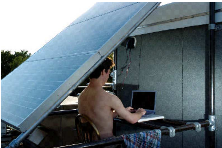
Fig. 3. Joshua Harris, project manager of the ETRC, is shown in the Solar Outdoor Labspace. The sun is directly powering the laptop computer which is connected to the solar panels by reconfigurable DC ‘banana jacks’.
