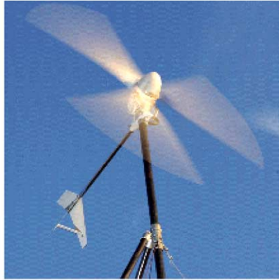
Fig. 5. The Urbine: Canada's first rooftop mounted urban wind turbine. The frame of the urbine also supported the outdoor shower, cooling occupants as they relax on the Flexible Solar Membrane.
