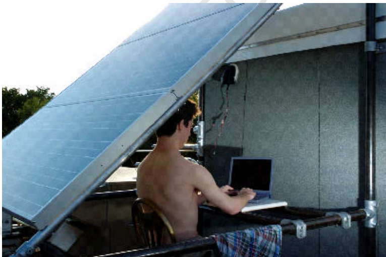
224 Fig. 3. Joshua Harris, project manager of the ETRC, is shown in the Solar Outdoor Labspace. The sun is directly 225 powering the laptop computer which is connected to the solar panels by reconfigurable DC ‘banana jacks’.
